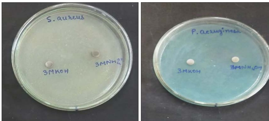
Fig 7: Zone of inhibition for (a) S.Aureus and (b) P.Aeruginosa shown by \text{Co}_3\text{O}_4 NPs synthesised with KOH and \text{NH}_4\text{OH}
